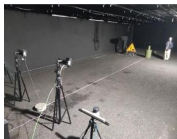
ARPA2 reception system characterization under harsh environmental conditions (fog, rain, night, dust)
